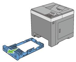
5 Lift the printer and align the five guide pins of the optional 250-sheet feeder with the holes at the bottom of the printer. Gently lower the printer onto the optional 250-sheet feeder.
